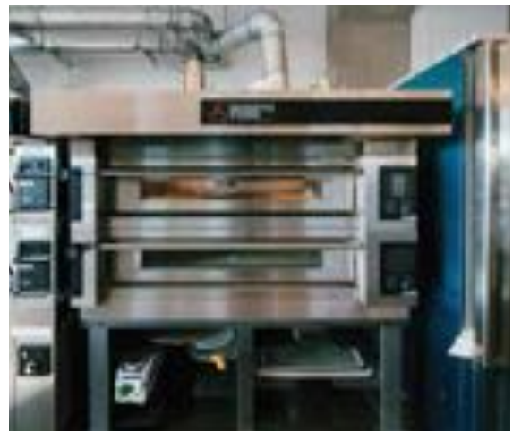
Moretti electric ovens from Faema Canada with refractory stone cooking plain & top and bottom heat sources. Photos: Rick O'Brien
