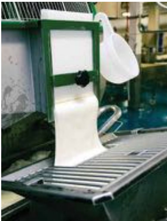
Curds heated, kneaded, extruded as pasta filter.
